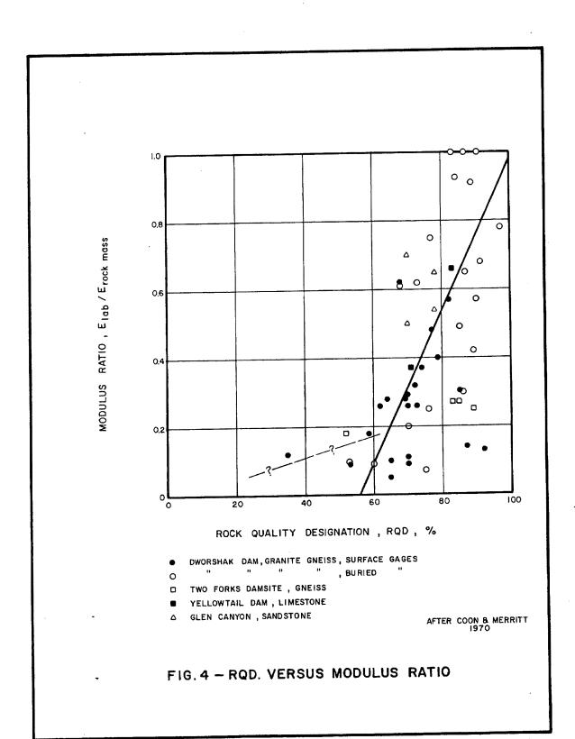
quite useful in evaluating the safety of existing concrete dams subject to loading from flood-overtopping, where the modulus of deformation of the foundation is required as an input factor.
