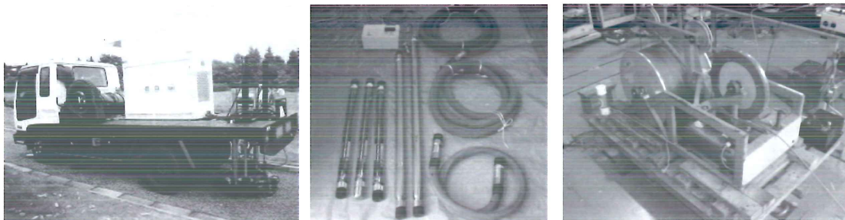
Fig.7. Field acquisition systems (Left: Minivib source, Middle: Borehole shuttle, Right: Winch).
